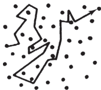
Figure 3.8 Zigzag path of a gas particle.
