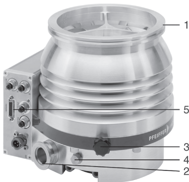
Figure 10.3 Single-flow turbomolecular pump HiPace 700 by Pfeiffer company with attached drive electronics for 48 V DC. 1: high-vacuum flange; 2: fore-vacuum flange; 3: venting valve; 4: purge-gas port; 5: electronic drive unit with remote control socket.
