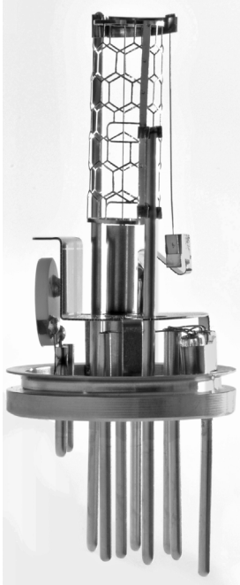
Figure 13.72 Combined vacuum gauge BCG 450 by INFICON with a range from 5 \times 10^{-8} Pa to 150 kPa. It is composed of a capacitive diaphragm sensor (left), a Pirani gauge (right), and an ionization gauge of the Bayard–Alpert type (center part). (Courtesy of INFICON AG , Liechtenstein.)
