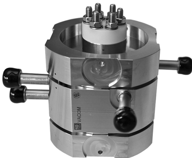
Figure 17.41 Resonant beam position monitor with electrical feedthrough.
