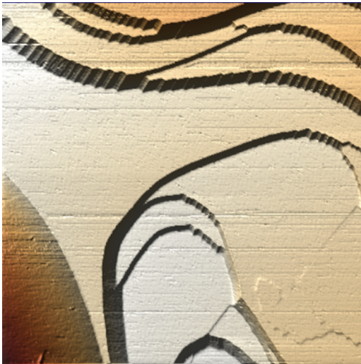
Figure 6.12 STM image of a vacuum fired stainless steel surface with (111) terraces and steps in between. The detail shows an area of 1 \mu\text{m} \times 1 \mu\text{m} . (By courtesy of M. Leisch, University Graz, Austria.)
