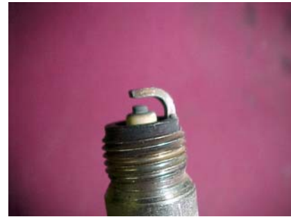
Figure 5. Non-Resistor Spark Plug After 97,000 Miles
