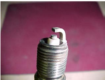
Figure 4. Non-Resistor Spark Plug After 56,000 Miles
