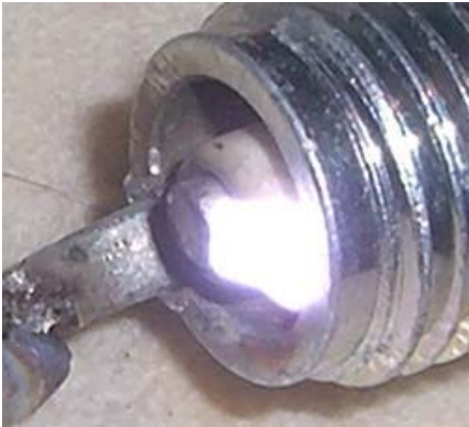
FIG 6.3 SURFACE GAP PLASMA HAS STRAP BUT I BENT IT BACK SO IT'S LIKE IT ISN'T THERE
