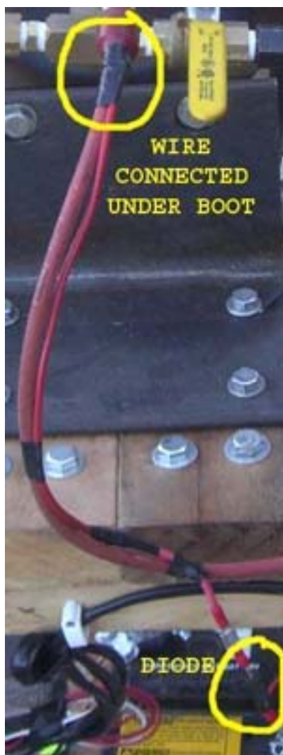
FIG 5.4 DIODE CONNECTED INSIDE OF BOOT
