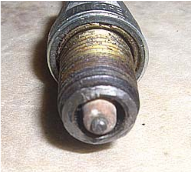
FIG 6.2 HOME MADE SURFACE GAP
